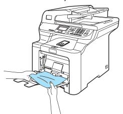
3 Close the MP tray. Then, open the front cover and close it to reset the machine. Open the MP tray again.
